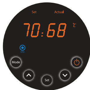
Temp. Display Interface The smart chip will show the setting and actual temperature of water
