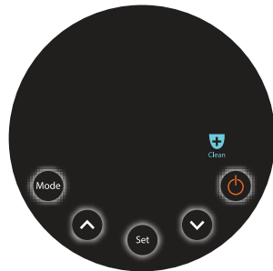
[Standby] Interface When the heater is not working for long and has gone into standby model
